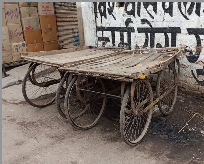
Unseasoned wood platform gets damaged easily
